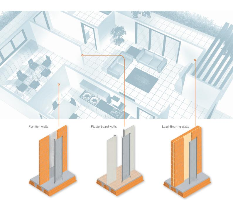
**NOTS:** for installation in bearing walls, make a 60 cm wide recess from floor to ceiling. For partition or plasterboard walls, leave an opening of approximately 60 cm during the construction of the wall.
