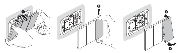
Removal of the control devices from the electrified frame for installation in a different position.
