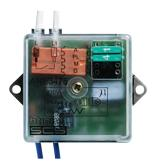
Actuator, item 3476 with 1 relay for single loads: 2 A resistive or incandescence lamps, 2 A inductive for ferromagnetic transformers. Preset for connection with NO type control pushbutton.
