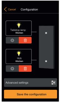
Customisation of the functions by the user - definition of the FULL command for the control of 2 separate light points.
