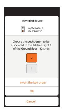
Activation of the MyHOME\_Up system definition of the LIGHT command for the control of two lights.
