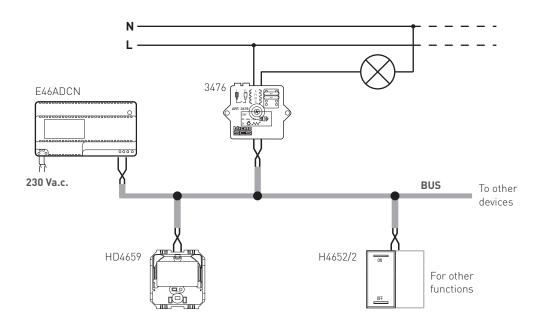
The device controls the load with the address indicated in A and PL. When a presence is detected, if the light level is below the set level the device switches on the assigned load and keeps it on for a period of time set using the configurator in T. The sensitivity of the PIR movement sensor is set using the configurator in S. For correct operation, it will be necessary to set the sensor lighting setpoint (see procedure).
