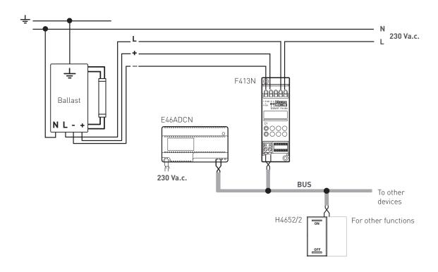
**DIAGRAM 6**SWITCHING ON, OFF AND ADJUSTMENT OF THE LIGHT LEVEL OF LED LAMPS
