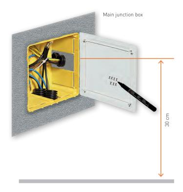
**NOTE:** For the installation of the boxes refer to the IEC 64-50 standard. The guide recommends a height from the floor exceeding 17.5 cm. We recommend approximately 30 cm.
