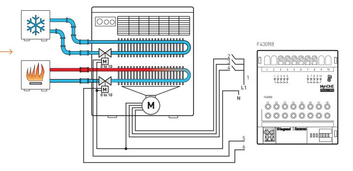
Variation for the connection of a 4-tube fan-coil with 0-10 V speed adjustment - use of two 0-10 V outputs (set LOAD = 3 in case of physical configuration).
