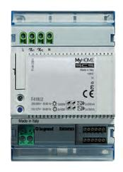
**ON/OFF actuator, item BMSW1003** with "Zero Crossing" technology, 4 independent outputs for 16 A maximum loads at 230 V a.c. The device is powered directly from the 100/240 Va.c. mains 50/60 Hz.
